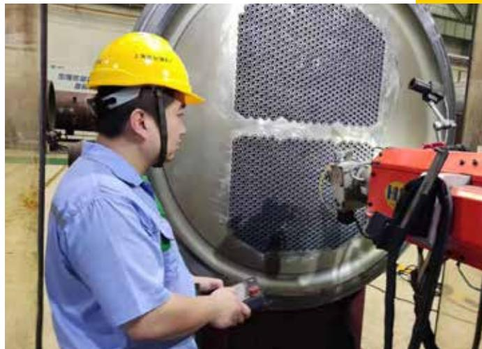
improvements on both the equipment and welding process parameters, they ultimately mastered the critical technology of internal bore welding, providing strong support for the welding manufacturing of the final product.
